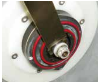
Curved Collet Wrench - the curve of the collet wrench enables you to reach the grooves on the spindle
