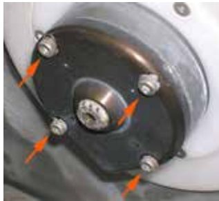
Spindle Cap A - four visible screws See "Spindle Cap A" on page 192
