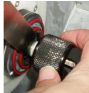
Use the wrench to hold the spindle in place while the collet tool turns the collet.
