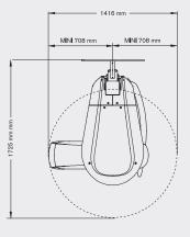
Minimum operational required space:\*\* Depth x width: 1725 mm x 1635 mm \*\*Refer to local regulatory requirements
